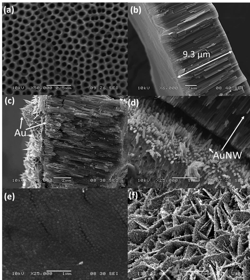
**Fig. 2** SEM images of pristine anodic  $\text{TiO}_2$  nanotube arrays after 20 minutes of 2<sup>nd</sup> step anodizing from (a) top view and (b) cross-section; and TNT–AuNW (c) cross-sectional view, (d) interface of AuNWs slightly detached from TNTs due to sample cutting, (e) top of the TNT–AuNW electrode (bottoms of TNTs), (f) flake-like morphology of its Au thin film (back side of the photoanode).
