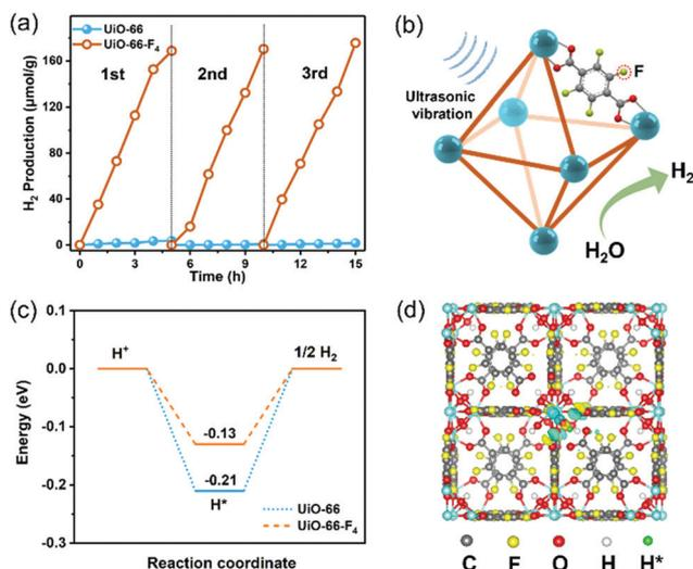
Fig. 4 (a) Three cycles of time-dependent H<sub>2</sub> evolution curves over UiO-66 and UiO-66-F<sub>4</sub> under ultrasonic vibration. (b) Schematic illustration of the mechanism of piezocatalytic H<sub>2</sub> production from water over the UiO-66-F<sub>4</sub> via harvesting vibration energy. (c) Gibbs free energy ( $\Delta G_{H^+}$ ) diagram for hydrogen adsorption on UiO-66 and UiO-66-F<sub>4</sub>. (d) Most stable atomic configurations of hydrogen adsorption on UiO-66-F<sub>4</sub>.
