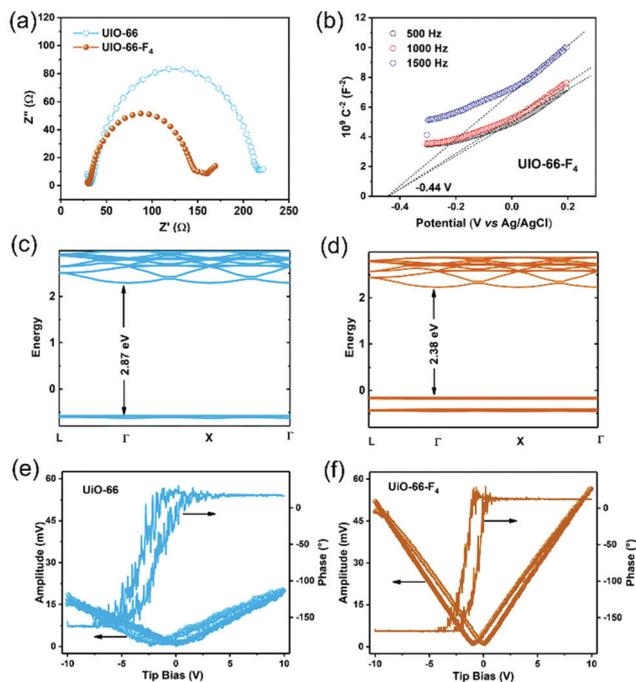
Fig. 3 (a) Electrochemical impedance spectra of UiO-66 and UiO-66-F<sub>4</sub>. (b) Mott–Schottky plots of UiO-66-F<sub>4</sub> at different frequencies. DFT calculation of the band structures of (c) UiO-66 and (d) UiO-66-F<sub>4</sub>. PFM phase and amplitude hysteresis loops of (e) UiO-66 and (f) UiO-66-F<sub>4</sub>.
