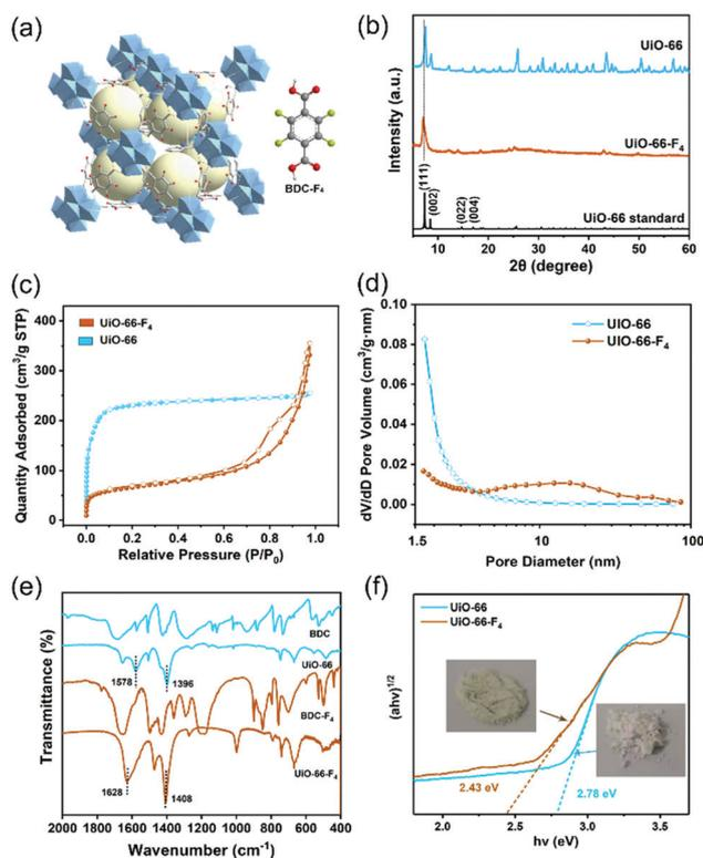
Fig. 2 (a) Crystal structure of the UiO-66-F<sub>4</sub> framework and H<sub>2</sub>BDC-F<sub>4</sub> linker. (b) XRD patterns, (c) Ar adsorption–desorption isotherms, (d) size distributions, (e) FTIR spectra, and (f) optical band gap calculation using Tauc's equation of UiO-66 and UiO-66-F<sub>4</sub>.
