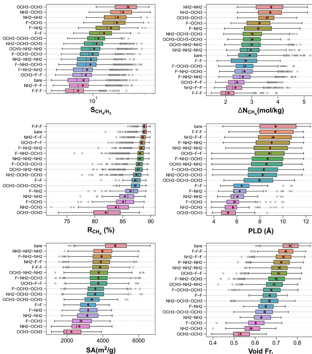
Fig. 4  $CH_4/H_2$  separation performance metrics and structural properties of MOFs classified by their functional groups.
