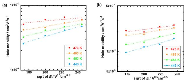
Fig. 4 Hole mobilities plotted for the square root of the electric field at various temperatures in the N\* phase of (a) compound **1** and (b) compound **2**.
