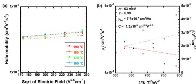
Fig. 7 (a) Hole mobilities plotted for the square root of the electric field at various temperatures in the N\* phase of the compounds **1–3** mixture (high temperature region). (b) Plots of zero-field mobility  $\mu_0$  and  $\beta$  as a function of the square of  $1/k_B T$  in the N\* phase of the LC mixture (high temperature region).
