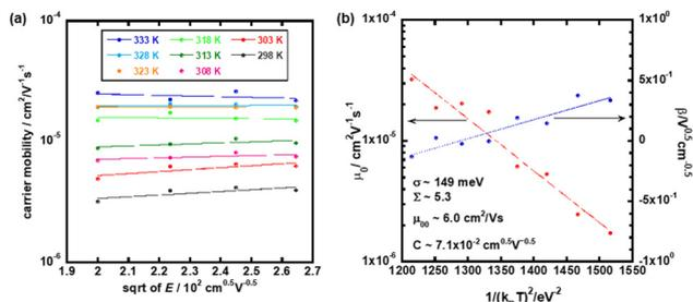
Fig. 8 (a) Hole mobilities plotted for the square root of the electric field at various temperatures in the N\* phase of the compounds **1–3** mixture (low temperature region). (b) Plots of zero-field mobility  $\mu_0$  and  $\beta$  as a function of the square of  $1/k_B T$  in the N\* phase of the LC mixture (low temperature region).
