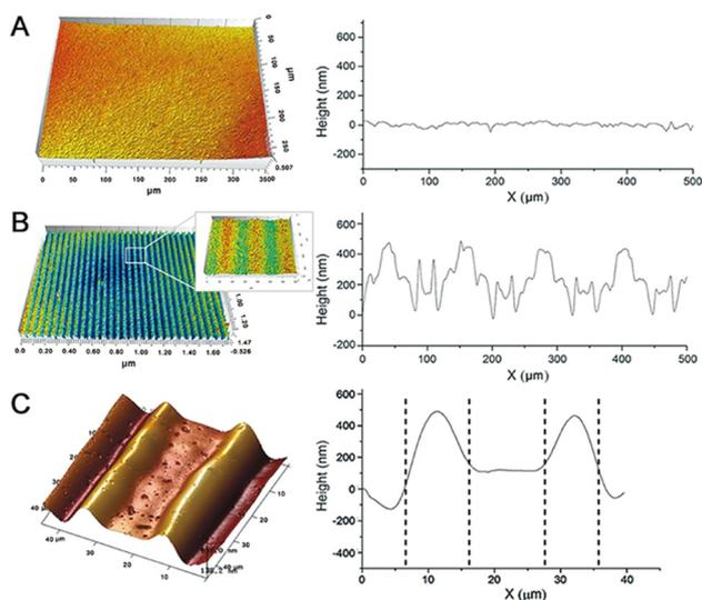
Fig. 3 Surface topographies and corresponding cross section curves of horizontally aligned fluorinated CLCP coating with a thickness of 5  $\mu\text{m}$  at 50  $^{\circ}\text{C}$  under an applied DC electric field of 100 V ( $E = 3.33 \text{ V } \mu\text{m}^{-1}$ ): 3D profiles before (A) and after electric actuation (B); AFM image after electric actuation (C). (3 cm  $\times$  3 cm ITO electrode substrate: gap, 30  $\mu\text{m}$ ; interval, 30  $\mu\text{m}$ ).
