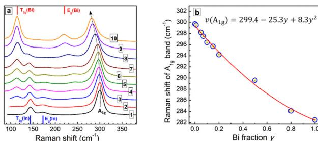
**Fig. 6** (a) Raman spectra of CANBIC perovskites with varied Bi fraction  $y = 0$  (1), 0.01 (2), 0.05 (3), 0.07 (4), 0.10 (5), 0.15 (6), 0.20 (7), 0.50 (8), 0.80 (9), and 1.00 (10). (b) Frequency of the  $A_{1g}$  mode as a function of Bi fraction  $y$  (scatter). Solid red line represents the best fit with a polynomial function “ $v(A_{1g})$  versus  $y$ ” presented in the figure.
