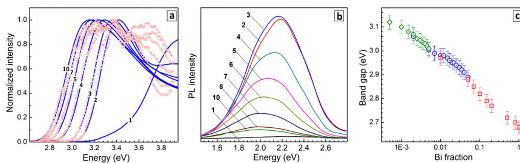
**Fig. 3** (a and b) Absorption, PL excitation (a), and PL (b) spectra of CANBIC perovskites with Bi fraction  $y = 0$  (curve 1), 0.01 (2), 0.05 (3), 0.07 (4), 0.10 (5), 0.15 (6), 0.20 (7), 0.50 (8), 0.90 (9), and 1.00 (10). In (a) solid lines are absorption spectra and circles represent corresponding PL excitation spectra. (c) Band gap of CANBIC perovskites as a function of Bi fraction  $y$ . A legend for different symbols in (c) is provided in the caption of Fig. 4.
