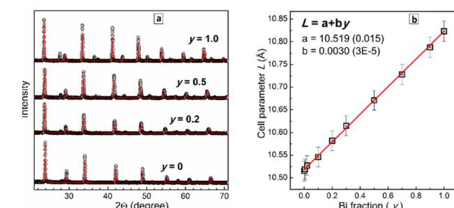
**Fig. 2** (a) X-Ray diffractograms of CANBIC perovskites with  $x = 0.4$  and  $y = 0, 0.2, 0.5$ , and  $1.0$ . Gray circles correspond to experimental data, red solid lines are the results of Rietveld refinement. (b) Cell parameter of CANBIC perovskites as a function of Bi fraction  $y$ . Gray squares are experimental data, red line represents a linear fit (fitting parameters  $a$  and  $b$  are presented in figure).
