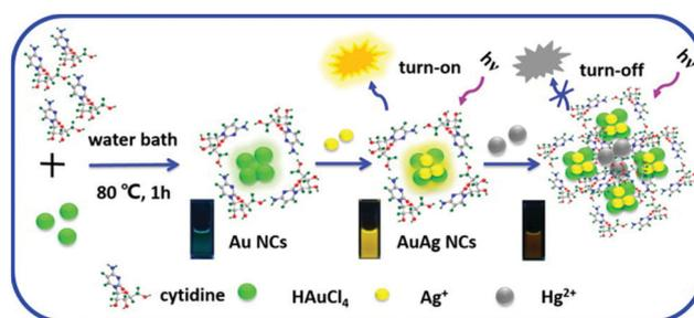
Fig. 12 Schematic illustration of the synthesis of cytidine-stabilised AuNCs and changes in the luminescence property with the addition of Ag<sup>+</sup> and Hg<sup>2+</sup>. Reproduced with permission from ref. 171, Copyright Elsevier (2015).
