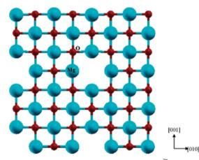
Fig. 5 Schematic representation of a Schottky defect<sup>71</sup> [Reprinted with permission. Copyright (2004) American Chemical Society].
