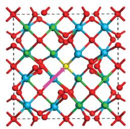
Fig. 4 General schematic of the formation path of a Frenkel pair defect (highlighted in pink) in La<sub>2</sub>Hf<sub>2</sub>O<sub>7</sub><sup>70</sup> [Reprinted with permission. Copyright (2017) American Chemical Society)
