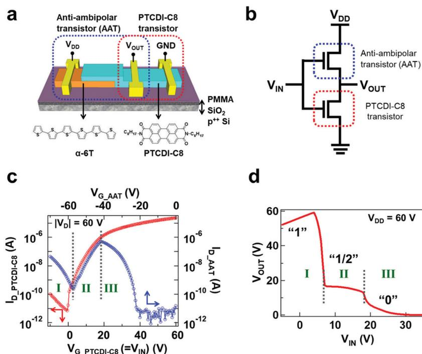
Fig. 8 (a) Illustration and (b) schematic diagram of an organic MVL circuit, where the  $\alpha$ -6T/PTCDI-C8 AAT and n-FET (PTCDI-C8) are connected in series. (c)  $I_D$ - $V_G$  curves for the n-FET (red) and AAT (blue). (d) Voltage transfer curve ( $V_{IN}$ - $V_{OUT}$ ), showing ternary inverter operation. Reprinted with permission from ref. 44 Copyright 2018 American Chemical Society.
