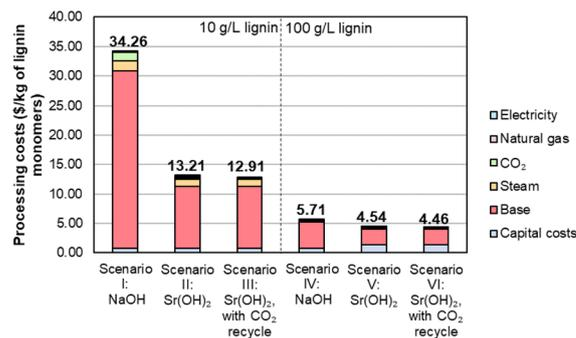
**Fig. 9** Economic analysis of lignin monomer production by alkaline oxidation promoted by  $\text{Sr}(\text{OH})_2$  compared to NaOH. Numerical data for this figure are included in Table S15.<sup>†</sup>
