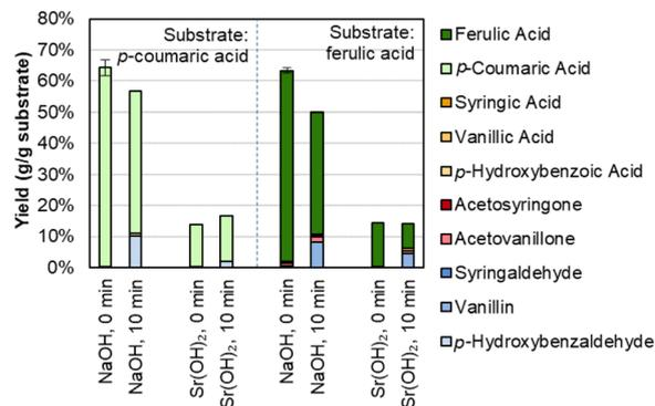
**Fig. 3** Recovery of *p*-coumaric acid and ferulic acid in the presence of NaOH or  $\text{Sr}(\text{OH})_2$ . Reaction conditions: 0.3 g *p*-coumaric (left four bars) or ferulic acid (right four bars), 30 mL water, 2 M hydroxide, 175 °C. For 10 min reaction times, air was added at reaction temperature to generate 30 bar total pressure (~22 bar air). Error bars represent the total monomer yield range of duplicate experiments. Numerical data for this figure are included in Table S2.†
