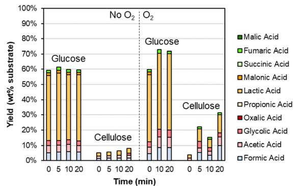
**Fig. 5** Degradation of carbohydrates during alkaline oxidation of lignin using  $\text{Sr}(\text{OH})_2$  as a reversibly soluble base. Reaction conditions: 0.3 g carbohydrate, 30 mL water, 1 M  $\text{Sr}(\text{OH})_2$ , 175 °C. For reactions with  $\text{O}_2$ , the reactor was pressurized to 30 bar total pressure with air when reactor reached 175 °C (~22 bar air). Numerical data for this figure are included in Table S7.†
