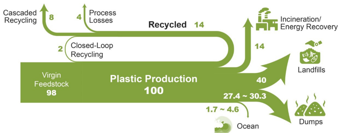
Fig. 1 Sankey Diagram showing the life cycle of plastic packaging. 5
