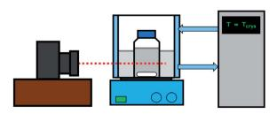
Fig. 2 Schematic representation of the experimental set-up.
