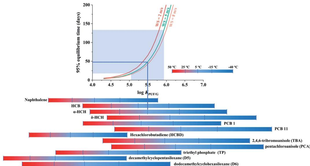
Fig. 4 Chart displaying the time to 95% equilibrium as influenced by chemical properties, temperature and wind speed. To use this plot, choose a target chemical and deployment temperature to get  $\log K_{\text{PUF/Gas}}$  on x-axis. Then deduce  $t_{95\%}$  on y-axis based on windspeed (e.g.  $t_{95\%}$  of 50 days for  $\alpha$ -HCH at 5 °C and 5  $\text{m s}^{-1}$ ).
