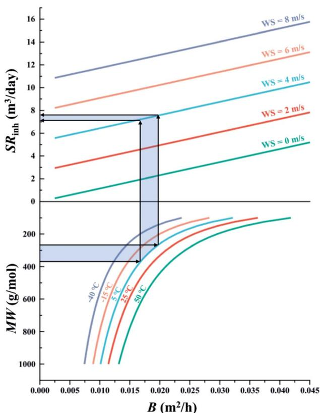
Fig. 2 Chart displaying the inherent sampling rate ( $\text{SR}_{\text{inh}}$ ) as a function of wind speed (WS) and a chemical's molecular diffusivity ( $B$ ), which in turn is a function of deployment temperature and the chemical's molecular weight (MW).
