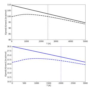
Fig. 7 Energy differences between products and reactant as a function of temperature in the harmonic approximation as obtained from Potentials A (upper panel) and C (lower panel). Full lines are classical values, while dashed lines are quantum ones. Vertical lines show the ZPE in K.
