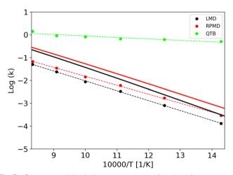
Fig. 3 Quantum and classical rate constants as a function of temperature for the 1-D Morse. In full lines we report values obtained from sum-ofstate approach (both classical and quantum), while results from trajectory simulations ( $\gamma = 0.01 \text{ fs}^{-1}$ ) are reported as dots: LMD (black), RPMD (red) and QTB (green).
