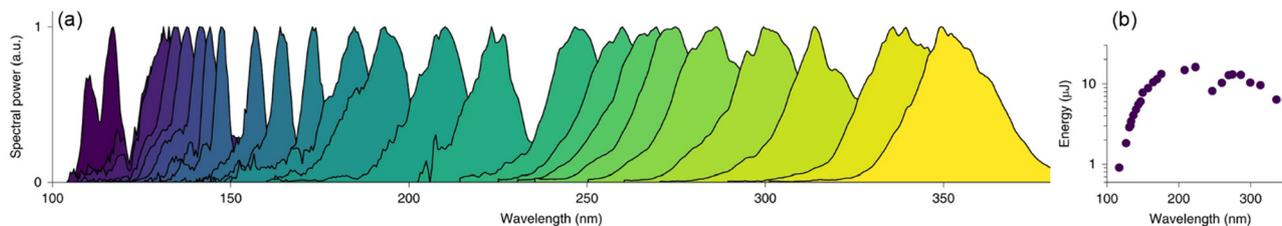
Fig. 11 Tunable RDW emissions in gas-filled HCFs. (a) Measured RDW spectra from a 3-m-long HCF with a 126  $\mu\text{m}$  core radius filled with helium and pumped with 10 fs pulses. (b) Measured pulse energies.<sup>84</sup> Adapted and reproduced with permission from Springer Nature.
