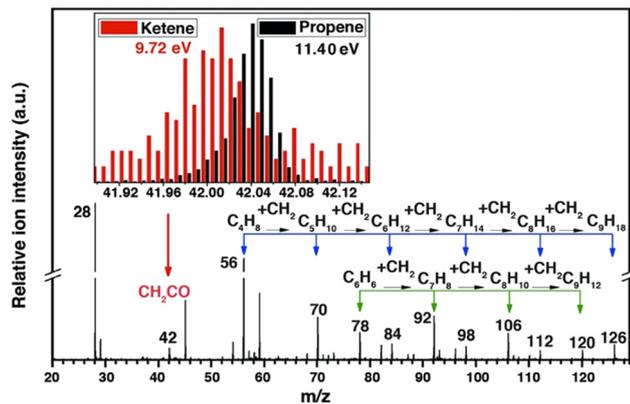
Fig. 9 Photoionization mass spectrum of products in syngas conversion over  $\text{ZnCrO}_x$  by SVUV-PIMS at 9.72 eV. The insets display the signals of  $m/z = 42.01$  (ketene) and  $m/z = 42.05$  (propene) detected at 9.72 and 11.40 eV, respectively.<sup>16</sup> Adapted and reproduced with permission from AAAS.
