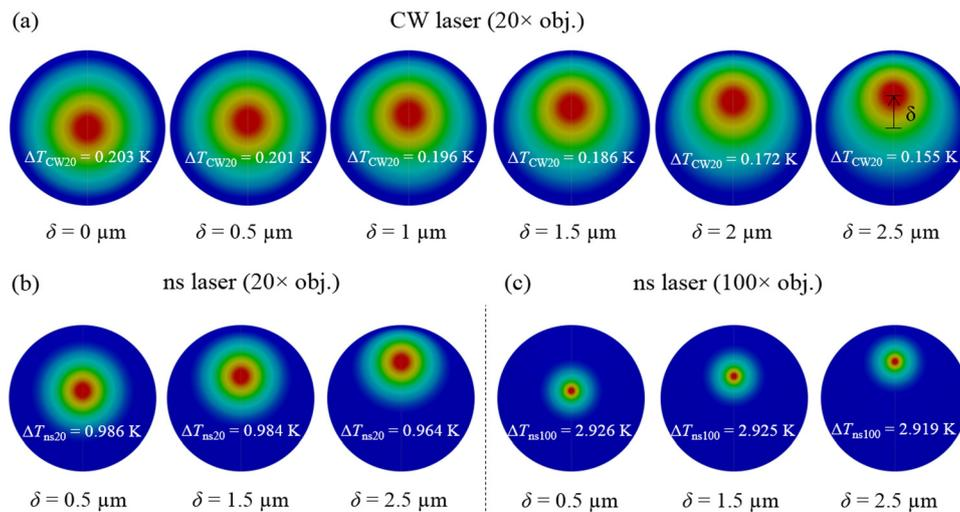
Fig. 10 Results of numerical analysis conducted by Zobeiri *et al.* to investigate the effect of laser spot position on the uncertainty of measured  $D$  of a suspended  $\text{WS}_2$  film. (a) CW laser heating ( $20\times$ ), (b) ns laser heating ( $20\times$ ), and (c) ns laser heating ( $100\times$ ). Reproduced from ref. 34 with permission from Elsevier, copyright 2019.
