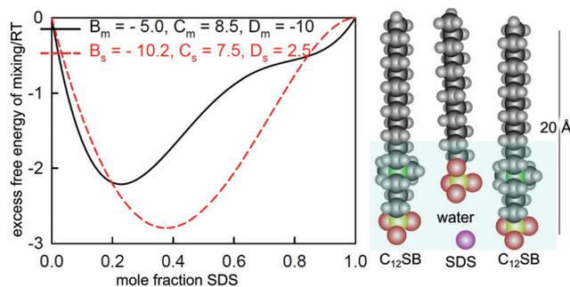
**Fig. 15** Dependence of the excess free energy of mixing for surface and micelles on the composition of SDS- $C_{12}SB$  mixtures, and a suggested molecular packing arrangement at the A-W interface. Redrawn from Li *et al.*<sup>126</sup>
