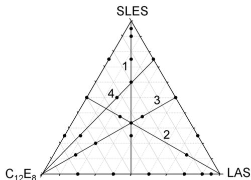
**Fig. 16** Ternary diagram for SLES/LAS/ $C_{12}E_8$  mixture, indicating the compositions at which NR measurements were made.
