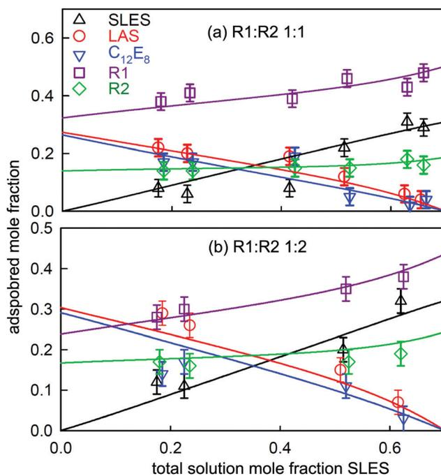
Fig. 18 Variation in adsorbed mole fraction for each component in the quinary mixture, SLES/LAS/ $C_{12}E_8$ /R1/R2, containing fixed mole fractions of R1 and R2. Reproduced by permission from Liley *et al.*<sup>113</sup>
