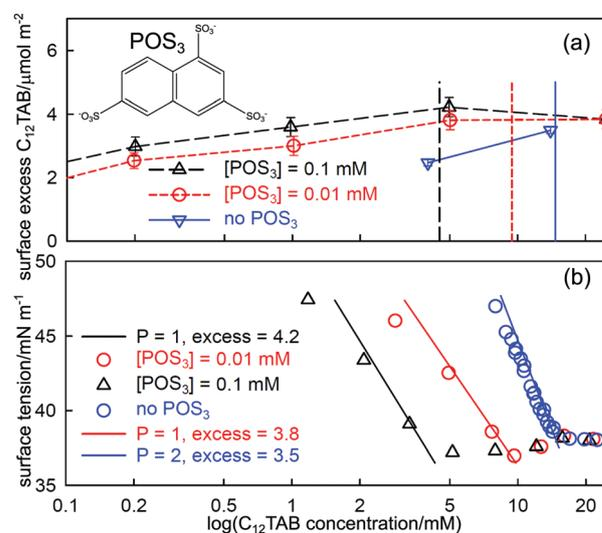
Fig. 5 (a) Surface excesses of  $\text{C}_{12}\text{TA}^+$  measured by NR at the A–W interface of  $\text{C}_{12}\text{TAB}$  on its own and with added amounts of 0.01 mM and 0.1 mM  $\text{POS}_3$  (trianion structure as shown in (a)), (b) the ST of the same set of solutions with fits of the integrated Gibbs equation using the prefactors and the surface excesses at the measured CMC given in the diagram, and the ST at the plateau. Data redrawn from Jiang *et al.*<sup>57</sup>
