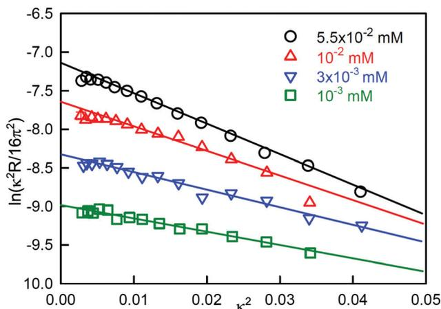
Fig. 1 Linear extrapolation of reflectivity data for  $C_{12}E_3$  solutions to obtain the surface excess at various concentrations using eqn (4). Data redrawn from Lu *et al.*<sup>1</sup>
