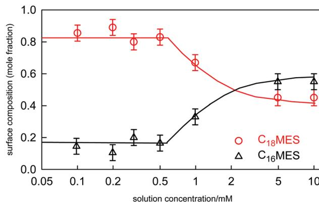
Fig. 10 Variation in surface composition with solution composition for the 65:35 mole ratio eutectic mixture of  $C_{16}$ MES/ $C_{18}$ MES. The lines are model calculations using the PPA with the parameters given in the text. Redrawn from Xu *et al.*<sup>114</sup>
