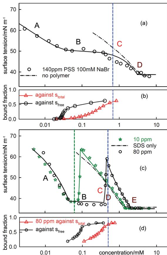
Fig. 7 The equivalent measurements to those in Fig. 6 but with electrolyte, (a)  $C_{12}$ TAB with NaPSS (MW = 18k) at a concentration of 140 ppm with 100 mM NaBr and (c) SDS with 10 ppm and 80 PDDA (MW = 100k) with 100 mM NaCl. The NR data are redrawn from ref. 69 and 70 and the binding isotherms redrawn from ref. 64 and 65.
