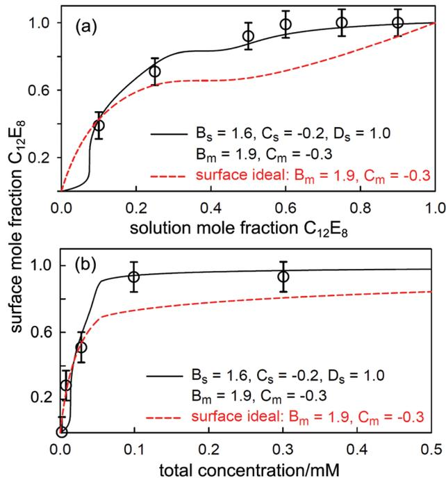
Fig. 13 (a) Variation in surface composition with solution composition at a solution concentration of 0.3 mM for escin/ $C_{12}E_8$ , (b) variation in surface composition with total surfactant concentration for 0.09 mM escin in  $C_{12}E_8$  solutions of varying concentration. The continuous lines are PPA calculations with non-ideal micellization and non-ideal surface mixing and the dashed lines are for non-ideal micellization and ideal surface mixing. Redrawn from Tucker *et al.*<sup>120</sup>
