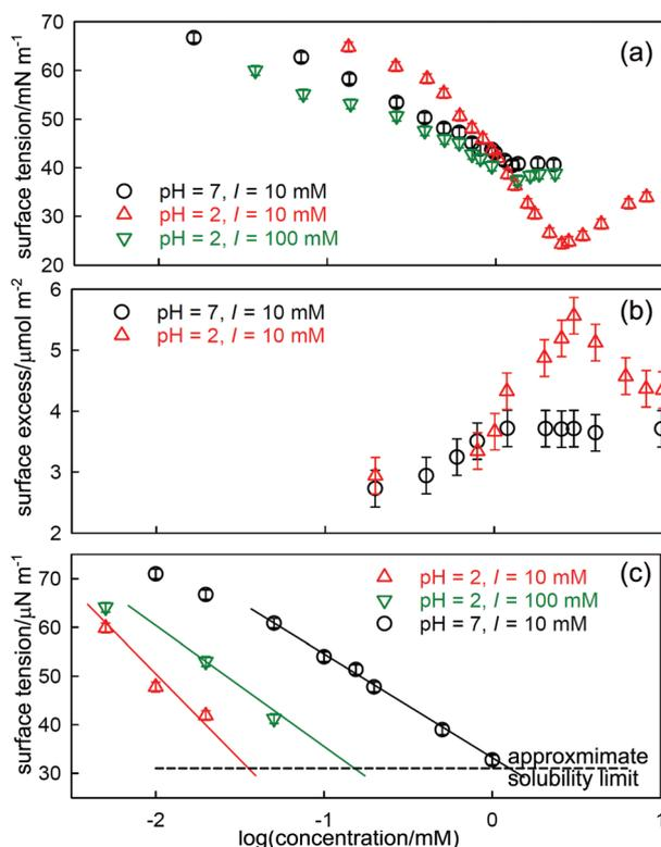
Fig. 2 Effects of hydrolysis of dodecanoyl-L-carnitine on its ST behaviour, (a) ST at pH of 2 and 7 and different ionic strengths ( $I$ ), (b) the total surface excess (dodecanoic acid and  $C_{12}CO_2LC$ ), and (c) the ST of dodecanoic acid at different pH. Data redrawn from Liu *et al.*<sup>23</sup>
