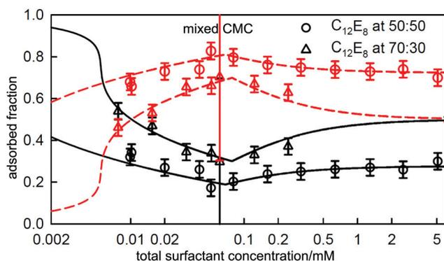
Fig. 11 Variation in surface composition with solution composition for  $C_{12}E_3:C_{12}E_8$  at 50:50 and 30:70 mole ratios. The lines are PPA calculations for  $B_m = -0.3$ ,  $B_s = 0.8$  and  $C_s = 1.2$ . Redrawn from ref. 20.
