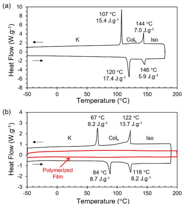
Fig. 2 DSC traces (second heating and cooling run) of (a) **HO-TTPSi<sub>3</sub>** and (b) **RM-TTPSi<sub>3</sub>** before (black trace) and after (red trace) photopolymerization at 25 °C. A temperature ramp of 10 K min<sup>-1</sup> was used. Exothermic heat flows have a positive value.
