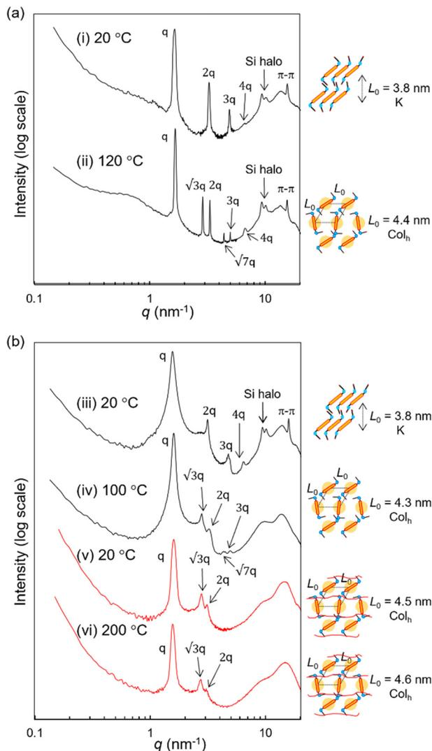
**Fig. 3** 1D transmission scattering profiles of (a) **HO-TTPSi<sub>3</sub>** and (b) **RM-TTPSi<sub>3</sub>** and schematic representations of the molecular packing. The black and red lines indicate a bulk and a film after photo-polymerization at 90 °C, respectively. The SAXS measurements were carried out at (i) 20 °C, (ii) 120 °C, (iii) 20 °C, (iv) 100 °C, (v) 20 °C and (vi) 200 °C.
