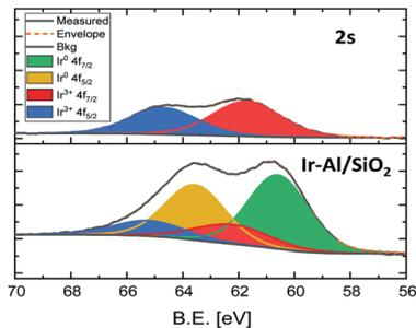
Fig. 3 XPS Ir 4f spectra of materials 2-s (top) and Ir-Al/SiO<sub>2</sub> (bottom).
