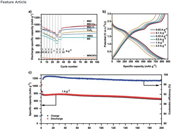
Fig. 6 (a) Galvanostatic rate performance test of all HESs, CoS<sub>2</sub>, 4MS2, and MWCNTs half-cell at different current densities and 25 °C in the voltage range between 0.01 and 3 V versus Li<sup>+</sup>/Li. (b) Voltage profiles of MS2 half-cell at different currents. (c) Specific charge/discharge capacity of MS<sub>2</sub> half-cell and Coulombic efficiency as a function of cycle number at 1 C and 25 °C in the range between 0.01 and 3 V. Copyright permission from Wiley, used from ref. 52
