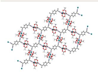
Fig. 10 WAQMEJ, a rhodium oxide based MOF which expands into 2-dimensional sheets. with a reported band gap of 0.71 eV (key: red -O, turquoise - Rh, grey - C, white - H, purple - N). The Cambridge Structural Database. 152
