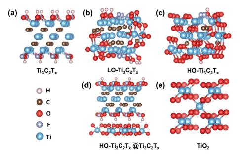
Fig. 5 Predicted crystal structures of Ti<sub>3</sub>C<sub>2</sub>T<sub>x</sub>, LO-Ti<sub>3</sub>C<sub>2</sub>T<sub>x</sub>, HO-Ti<sub>3</sub>C<sub>2</sub>T<sub>x</sub>, HO-Ti<sub>3</sub>C<sub>2</sub>T<sub>x</sub> and TiO<sub>2</sub> carried out by VASP code based on DFT.
