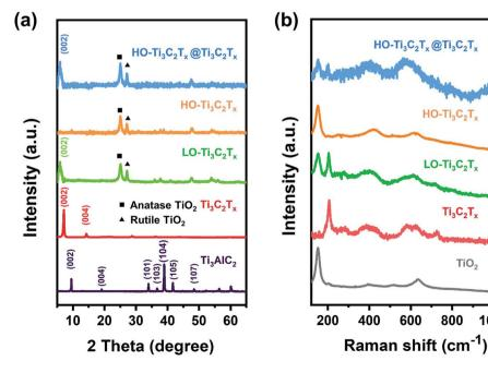
Fig. 2 (a) XRD patterns of  $Ti_3AlC_2$  powder and the dried films of  $Ti_3C_2T_x$ ,  $LO-Ti_3C_2T_x$ ,  $HO-Ti_3C_2T_x$ ,  $HO-Ti_3C_2T_x$ @ $Ti_3C_2T_x$ . (b) Raman patterns of  $Ti_3C_2T_x$ , LO- $Ti_3C_2T_x$ , HO- $Ti_3C_2T_x$ , HO- $Ti_3C_2T_x$ @ $Ti_3C_2T_x$  and  $TiO_2$  films.
