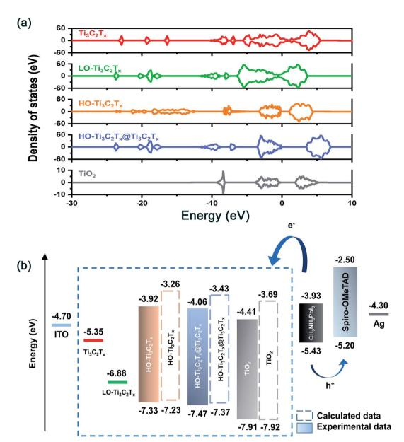
Fig. 6 (a) Calculated density of states for Ti<sub>3</sub>C<sub>2</sub>T<sub>x</sub>, LO-Ti<sub>3</sub>C<sub>2</sub>T<sub>x</sub>, HO-Ti<sub>3</sub>C<sub>2</sub>T<sub>x</sub>, HO-Ti<sub>3</sub>C<sub>2</sub>T<sub>x</sub>, TiO<sub>2</sub> and (b) schematic diagram of devices' each layer based on different ETLs determined by DFT calculation and UPS data.
