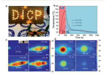
(a) LED lights of "DICP" characters with FCA2-C20, (b) electrothermal conversion curves and (c and d) infrared imaging pictures of the electro-thermal conversion process of FCA2-C20.
