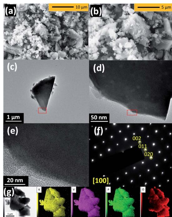
Fig. 2 (a and b) SEM and (c–e) TEM images, (f) SAED pattern, and (g) TEM-EDX mapping of as-prepared  $K_6(\text{VO})_2(\text{V}_2\text{O}_3)_2(\text{PO}_4)_4(\text{P}_2\text{O}_7)$ . (b) Magnified SEM image of the panel 'a'. (d) and (e) Magnified TEM images of the red square area represented in the panel 'c' and 'd', respectively.
