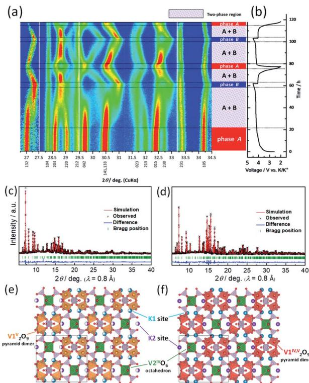
Fig. 7 (a) Contour map of *operando* XRD patterns in selected  $2\theta$  regions and identified phase regions. (b) Charge–discharge profiles during the *operando* XRD measurement. *Ex situ* synchrotron XRD patterns of the KVPP electrodes (c) charged to 4.5 V and (d) discharged to 2.0 V. (e and f) Refined crystal structures by Rietveld method for the XRD patterns shown in panel ‘c’ and ‘d’, respectively.
