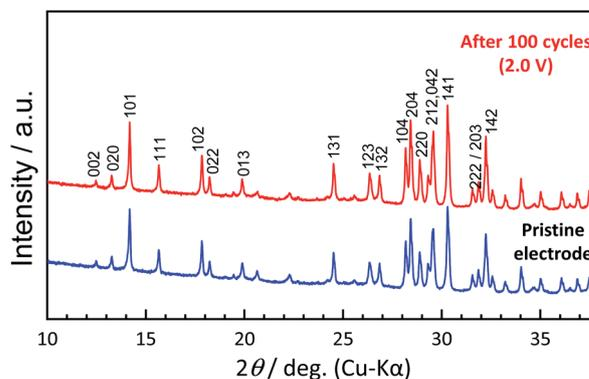
Fig. 4 Comparison of XRD patterns of pristine KVPP electrode and the KVPP electrode in the discharged state at 2.0 V at the 100<sup>th</sup> cycle.
