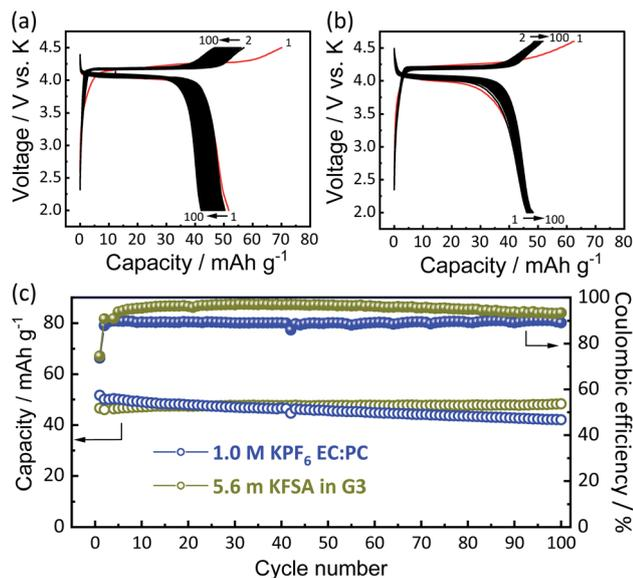
Fig. 5 Galvanostatic charge–discharge curves of KVPP electrodes in K cells filled with different electrolytes at C/20 rate in 2.0–4.5 V: (a) 1 mol dm<sup>-3</sup> KPF<sub>6</sub>/EC : PC (1 : 1 v/v) electrolyte and (b) 5.6 mol kg<sup>-1</sup> KFSA/triglyme (G3) electrolyte. (c) Comparison of discharge capacity and coulombic efficiency of the two different electrolyte cells.
