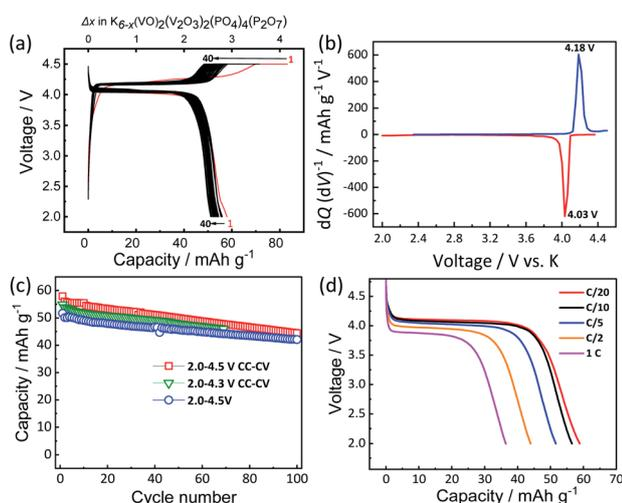
Fig. 3 Electrochemical properties of KVPP: (a) charge–discharge profiles for the first 40 cycles at C/20 current rate in the potential range of 2.0–4.5 V (with constant voltage step at 4.5 V), (b)  $dQ/dV$  plot of the second charge–discharge profile, (c) capacity retention plots of KVPP at C/20 rate in different voltage windows and (d) discharge profiles of KVPP at different current rates on the discharging process.
