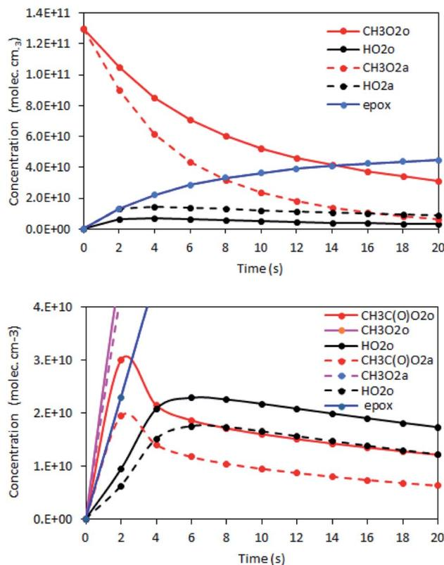
Fig. 3 Examples of simulations of the  $RO_2 + \text{alkene}$  reactions, showing the concentration profiles in the reactor for  $RO_2$  (red and pink),  $HO_2$  (black), and epoxy products (blue). The solid lines are the profiles in the absence of alkenes and the dashed ones in the presence of alkenes. Top:  $CH_3O_2 + \text{isoprene}$  reaction (experiment Alk05); bottom:  $CH_3C(O)O_2 + \text{isoprene}$  reaction (experiment Alk31).
