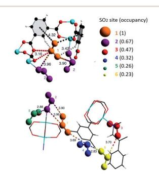
Fig. 1 SO<sub>2</sub> positions within MFM-170 pores obtained from in situ single-crystal X-ray diffraction. Purple SO<sub>2</sub> molecule is located at the thermodynamically strongest binding site. Cu, cyan; C, black; O, red; N, blue. Reprinted (adapted) with permission from ref. 19. Copyright (2019) Springer Nature.
