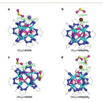
Fig. 6 DFT structure minimization of molecular configuration of one (a and b) and two (c and d) adsorbed SO<sub>2</sub> molecules on 1@KOH (left) and 1@Ba(OH)2 (right) materials. For sake of clarity, only the region around the metal cluster is shown. Ni (cyan); K (purple); Ba (wine); C (grey); N (blue); O (magenta); H (white); S (yellow). Reprinted (adapted) with permission from ref. 45. Copyright (2017) Springer Nature.
