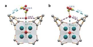
Fig. 3 Binding sites for  $SO_2$  molecules within MFM-300(In) determined by single-crystal X-ray diffraction (a), and DFT calculations (b). Reprinted (adapted) with permission from ref. 37b. Copyright (2016) John Wiley & Sons.
