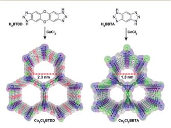
Fig. 17 Structure of  $Co_2Cl_2$  BTDD (left) and  $Co_2Cl_2$  BBTA (right). C, gray; O, red; N, blue; Cl, green; Co, purple. Hydrogen atoms have been omitted for clarity. Reprinted with permission from ref. 108. Copyright (2018) American Chemical Society.
