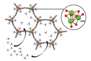
Fig. 18 Atomic structure of  $M_2$ (dobpdc) complexes with one-dimensional hexagonal channels. It is possible to observe that each coordinatively unsaturated metal site points towards the channel Reprinted (adapted) with permission from ref. 109. Copyright (2020) John Wiley & Sons.
