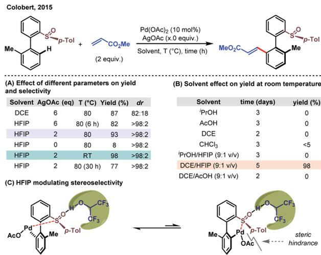
Scheme 15 Pd(II)-catalyzed atroposelective olefination of biaryls. (A) Overall optimization of the reaction; (B) effects of different solvents at room temperature on yield; and (C) steric induction by HFIP favoring one diastereoisomer.
