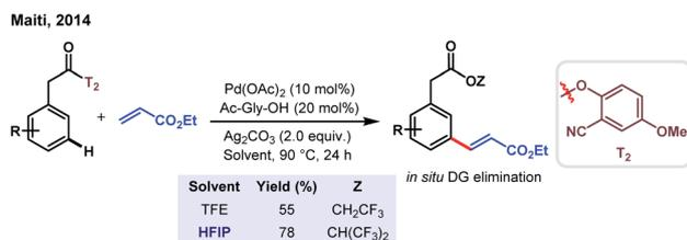
Scheme 6 Remarkable solvent effect by HFIP in Pd(II)-catalyzed *meta*-C(sp<sup>2</sup>)-H olefination of aryl acetic acids.
