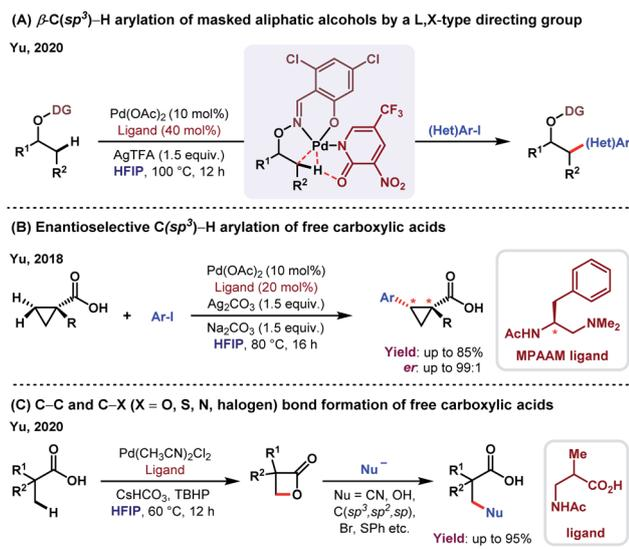
Scheme 4 Pd-Catalyzed β-C(sp<sup>3</sup>)-H functionalization using HFIP as the key solvent.
