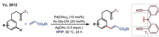
Scheme 5 First instance of Pd(II)-catalyzed *meta*-C(sp<sup>2</sup>)-H olefination of hydrocinnamic acids in HFIP medium.
