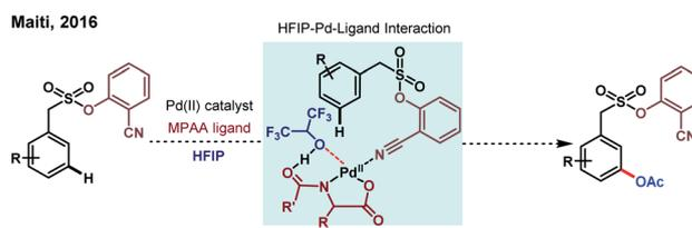
Scheme 7 HFIP-Pd-ligand interaction in Pd(II)-catalyzed *meta*-C(sp<sup>2</sup>)-H acetoxylation of aryl sulfonamides.
