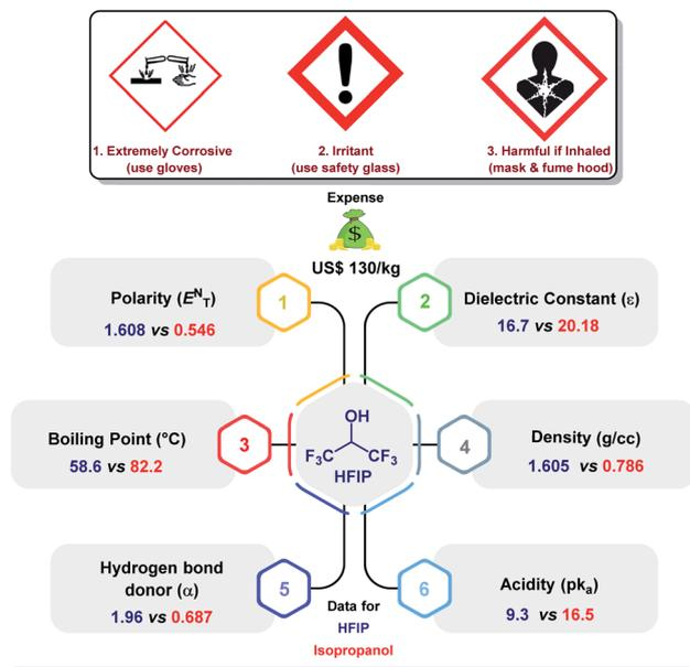
Fig. 1 A comparative overview of different physical characteristics, price, and safety details of HFIP and isopropanol.<sup>20,21</sup>
