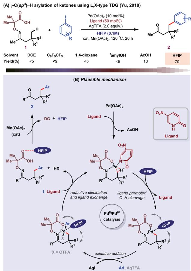
Scheme 14 (A)  $\gamma$ -C(sp<sup>3</sup>)-H arylation of ketones; (B) mechanistic blueprint displaying the detailed role of HFIP.
