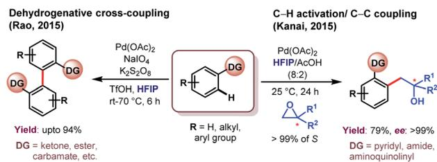
Scheme 3 Pd-catalyzed C(sp<sup>2</sup>)-H bond functionalization reactions.
