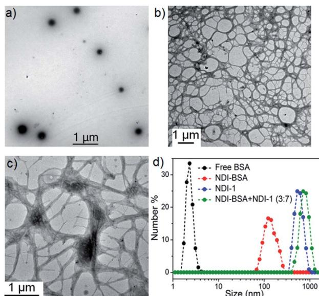
Fig. 2 TEM images of (a) NDI-BSA, (b) NDI-1 and (c) NDI-BSA + NDI-1 (3 : 7); (d) number averaged size distribution of BSA, NDI-BSA, NDI-1 and NDI-BSA + NDI-1 (3 : 7) from DLS measurements ( $c = 0.05$  mM in all samples). Autocorrelation function corresponding to the DLS plots are shown in the ESI (Fig. S6<sup>†</sup>).
