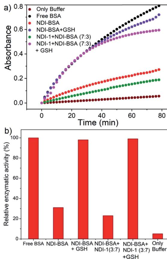
Fig. 4 (a) Time dependent change in absorption of *p*-nitro phenol ( $\lambda = 405$  nm) produced by hydrolysis of the NPA substrate with BSA in different forms as indicated in the figure.  $T = 25$  °C; concentration of BSA and NPA = 0.1 mM and 10 mM, respectively; (b) relative enzymatic activity of BSA in different samples as estimated from the slope of each curve for the first 20 minutes and assuming free BSA activity as 100%.
