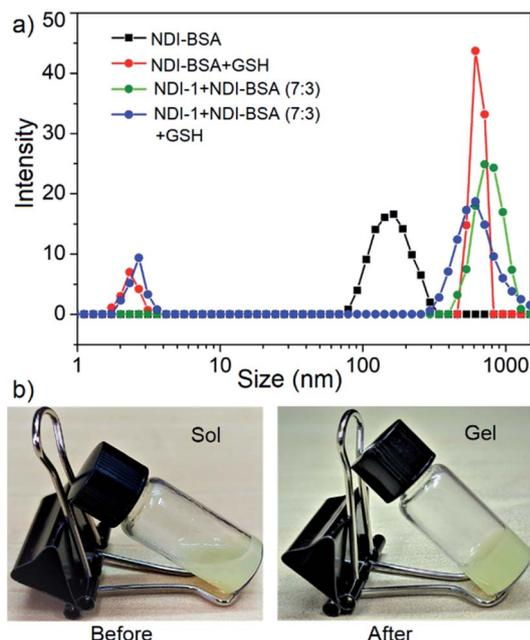
Fig. 5 (a) DLS profile NDI-BSA and NDI-1 + NDI-BSA (7 : 3) before and after GSH (1.5 mM) treatment.  $c = 0.05$  mM. Autocorrelation function corresponding to the DLS plots are shown in the ESI (Fig. S11†); (b) image of aqueous solution of NDI-1 + NDI-BSA (7 : 3) ( $c = 5.0$  mM) before and after treatment with GSH (10.0 mM) and gentle heating.
