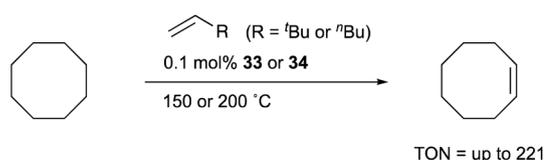
Scheme 13 Catalytic dehydrogenation using the PBP–Ir complexes 33 and 34.
