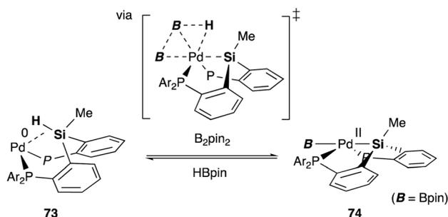
Scheme 33 Reversible  $\sigma$ -bond metathesis of the  $\eta^2$ -(Si–H)Pd<sup>0</sup> complex **73** with B<sub>2</sub>pin<sub>2</sub>.
