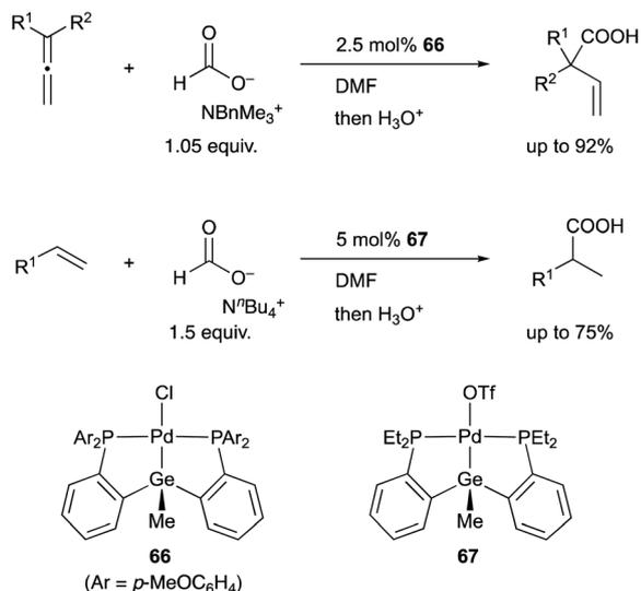
Scheme 30 PGeP–Pd complex **66** or **67**-catalyzed hydrocarboxylation using a formate salt as both a reductant and CO<sub>2</sub> source.
