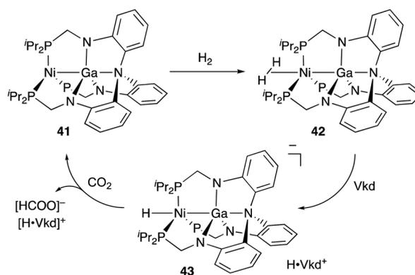
Scheme 17 Catalytic hydrogenation of CO<sub>2</sub> using the Ni-Ga complex 41.
