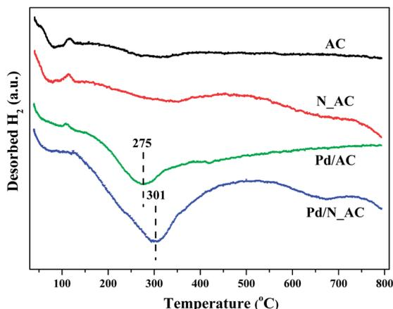
Fig. 5 H<sub>2</sub>-TPD profiles of AC, N\_AC, Pd/AC and Pd/N\_AC.
