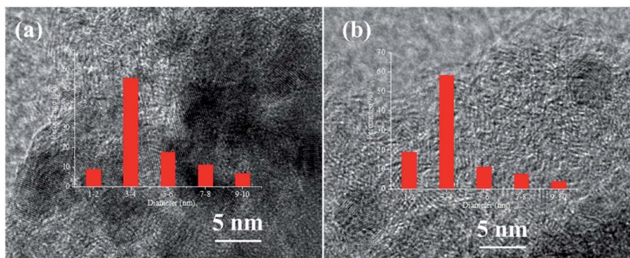
Fig. 4 HRTEM images and size distribution of (a) Pd/AC and (b) Pd/N<sub>AC</sub>.
