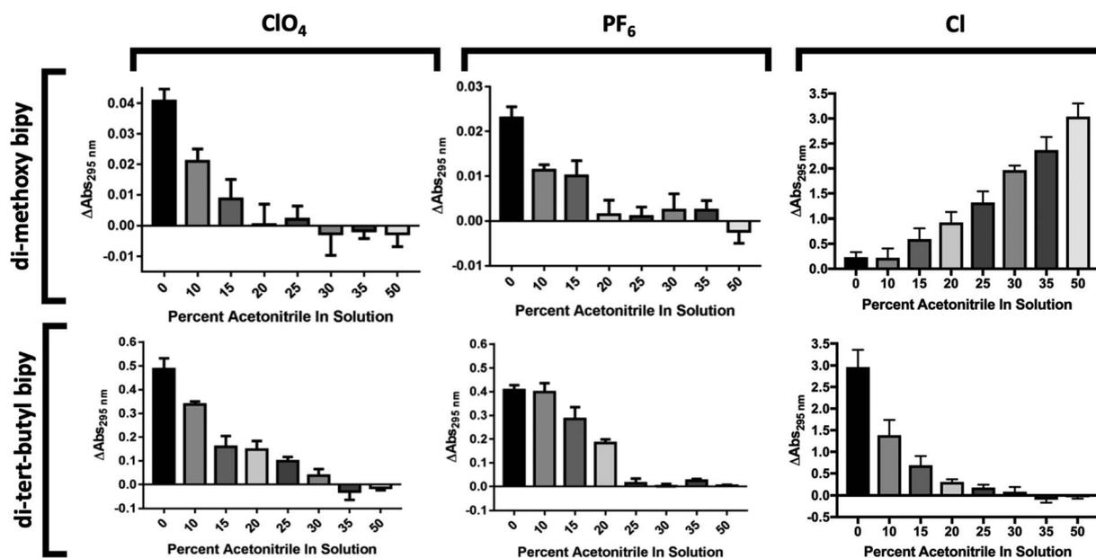
Fig. 5 Solubility of cobalt redox mediators in acetonitrile : H<sub>2</sub>O binary solvent systems. The solubility of all six complexes in increasing percentages of acetonitrile was assessed to determine minimum concentration of acetonitrile needed for solubility. All samples were chemically oxidized prior to measurement. Error bars represent SEM.
