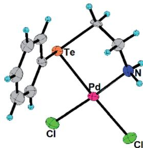
Fig. 1 ORTEP diagram of complex 1 with 50% thermal ellipsoids. Selected bond lengths (Å): Te–Pd: 2.5057(6), Te–C<sub>aryl</sub>: 2.118(6), Te–C<sub>alkyl</sub>: 2.149(6), Pd–Cl: 2.3142(16), Pd–Cl; Pd–N: 2.063(5). Selected bond angles (°): Cl–Pd–Te: 88.82(4), Cl–Pd–Cl: 94.42(6), N–Pd–Te: 88.21(13), N–Pd–Cl: 88.54(14).
