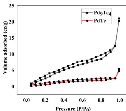
Fig. 10 N<sub>2</sub> adsorption–desorption isotherm of Pd<sub>9</sub>Te<sub>4</sub> and PdTe nanostructures.
