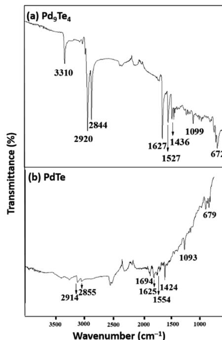
Fig. 4 FTIR spectra of (a) Pd<sub>9</sub>Te<sub>4</sub> (b) PdTe nanostructures.
