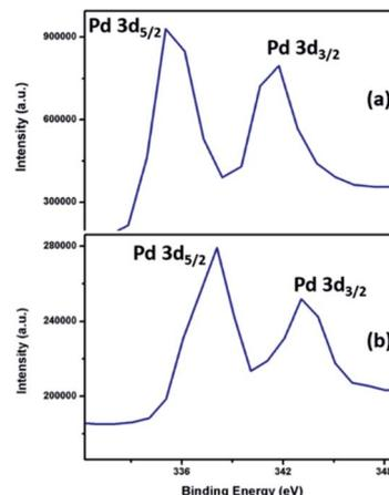
Fig. 9 XPS spectra of (a) Pd<sub>9</sub>Te<sub>4</sub> and (b) PdTe nanostructures.
