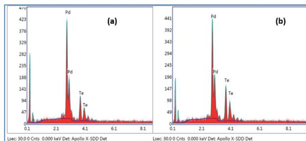
Fig. 6 SEM-EDS spectra of (a) Pd<sub>9</sub>Te<sub>4</sub> (b) PdTe nanostructures.
