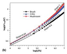
Fig. 10 Mean square displacement of membranes: (a) 2 dimensions MSD as a function of time for DPPC molecules (the component of MSD in the z-direction is neglected), (b) log-log of MSD as a function of time for DPPC molecules.
