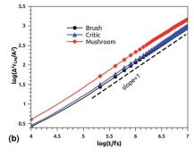
Fig. 11 Mean square displacement of confined ions: (a) 3 dimensions MSD as a function of time, (b) log-log of MSD as a function of time.
