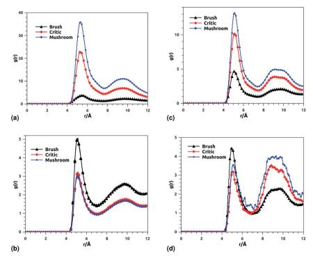
Fig. 8 RDF of membrane grafted chitosan components: (a) RDF of the group of chitosan molecules, (b) RDF of the group of lipid molecules, (c) RDF of the group of (chitosan molecules + lons), (d) RDF of the group of ions.
