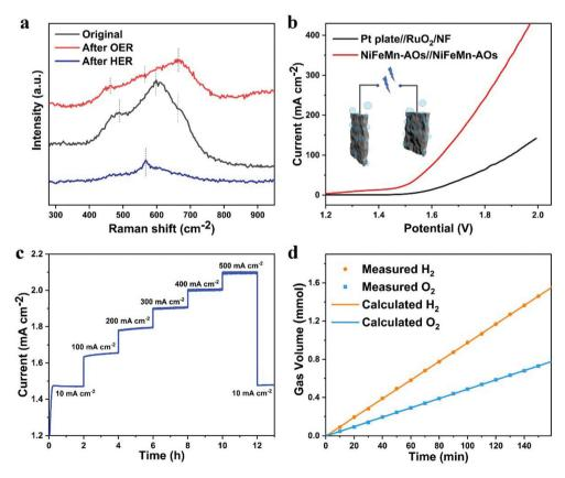
Fig. 5 (a) Raman spectra of the NiFeMn-AOs sample. (b) Polarization curves of NiFeMn-AOs//NiFeMn-AOs and Pt plate//RuO2 electrolyzer (without iR-compensation). (c) Chronopotentiometry curves of NiFeMn-AOs/NiFeMn-AOs at various current densities. (d) The volumes of H2 and O2 experimentally measured at 100 mA cm<sup>-2</sup>.
