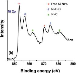
Fig. 8 XPS analysis of the Ni-rGO-zeolite composite catalyst after the first run: (a) survey scan and (b) high resolution Ni2p spectrum.
