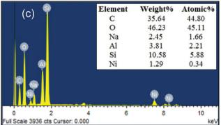
**Fig. 5** SEM images of (a) GO–zeolite, (b) Ni–rGO–zeolite, and (c) representative EDS spectrum of Ni–rGO–zeolite, elemental composition is shown in the inset (average values of 3 sets of EDS data).
