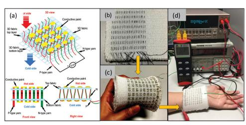
Fig. 15 (a) Systematically structured design of TEG based on 3D fabric, (b) yarn legs embroidered into the spacer fabric matrix, (c) flexibility of the fabricated prototype fabric TEG, (d) image showing the conversion of body heat into output power using the prototype TEG. Reprinted with permission from ref. 160 (Q. Wu, J. Hu, Smart Mater. Struct. 26 (2017) 045037). Copyright (2017), IOP Science Publications.
