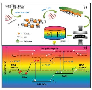
Fig. 16 (a) Schematic representation of the preparation of RGO-CdS-PANI nanocomposites for thermoelectric applications and (b) graphical representation of the energy levels of RGO-CdS-PANI nanocomposite promoting p-type charge transport and energy filtering effect. Reproduced from ref. 165 with permission from RSC Publications, Copyright 2017.
