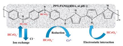
Fig. 8 Schematic representation of possible Cr(vi) adsorption by PPY-PANI@RHA
