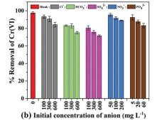
Fig. 7 Effect of co-existing (a) cations, (b) anions on the removal of  $Cr(v_1)$  by **PPY-PANI@RHA**. (Initial  $Cr(v_1)$  concentration: 50 mg  $L^{-1}$ ; contact time: 300 min; agitation speed: 200 rpm; pH  $\sim$  2; temperature: 303 K).
