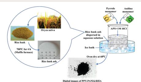
Fig. 1 Schematic representation of the synthesis process of polyprrole-polyaniline coated rice husk ash.
