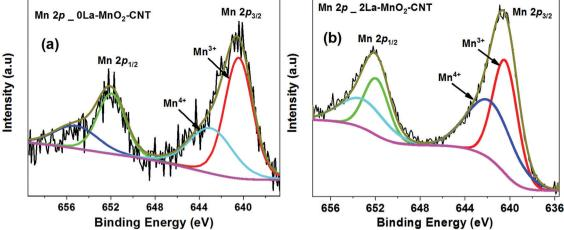
Fig. 3 XPS spectra of Mn 2p of OLa-MnO<sub>2</sub>-CNT (a) and 2La-MnO<sub>2</sub>-CNT (b).
