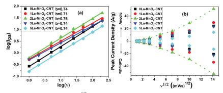
Fig. 8 log of peak current ( $I_{pc}$ ) vs. log(v) plot (a); and  $I_{pc}$  vs.  $v^{1/2}$  plot (b) of all the samples.
