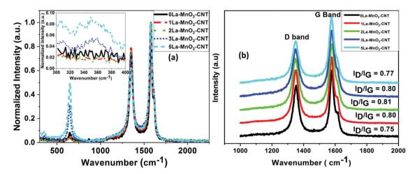
Fig. 2 Raman spectra of undoped and La-doped  $MnO_2$ -CNT (a); Raman spectra showing the D band and G band of undoped and La-doped  $MnO_2$ -CNT (b).
