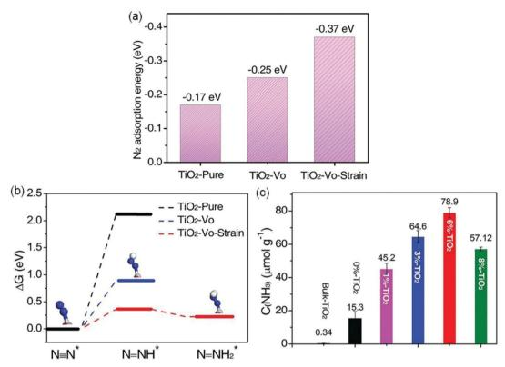
Fig. 8 (a) The  $N_2$  adsorption energies by DFT calculations on different photocatalysts. (b) The calculated Gibbs free energy for  $N_2$  reduction on the (001) surface of different photocatalysts (H: white sphere, Ti: gray sphere, N: blue sphere, O: red sphere). (c) Yield of  $NH_3$  over various samples under UV-vis irradiation. Reproduced from ref. 68 with permission from Wiley-VCH.
