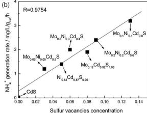
Fig. 6 (a) The  $N_2$ -TPD of  $Mo_{0.1}Ni_{0.1}Cd_{0.8}S$  and  $Mo_{0.1}Ni_{0.1}Cd_{0.8}S$ . (b) The relationship of  $NH_3$  yield over the obtained photocatalysts and the SV concentration. Reproduced from ref. 57 with permission from The Royal Society of Chemistry.
