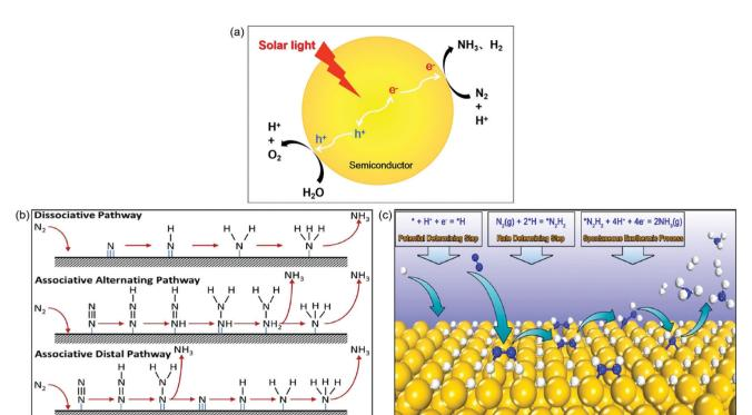
Fig. 1 (a) Photocatalytic synthesis of NH<sub>3</sub> in water. (b) The proposed mechanisms for photocatalytic N<sub>2</sub> reduction consisting of the dissociative pathway, the associative alternating pathway, and the associative distal pathway. Reproduced from ref. 27 with permission from ACS Publication. (c) The proposed mechanism of surface-hydrogenation over noble metal doped photocatalysts for NRR. Reproduced from ref. 28 with permission from ACS Publication.
