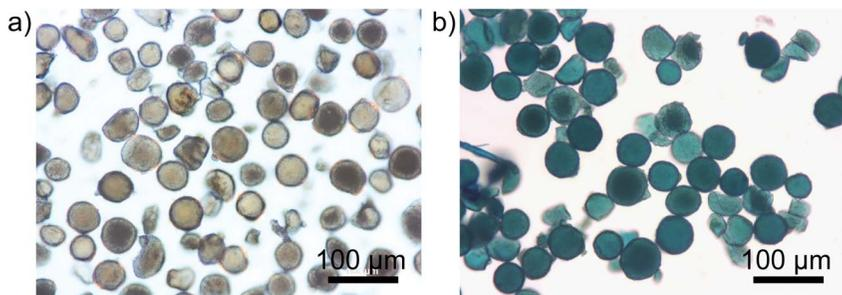
Fig. 6 Two optical images of Pd/SiO<sub>2</sub> before (a) and after (b) adding them to 20 ppm methylene blue (MB) in ethanol. The blue color is caused by adsorption of MB on the surface of the solid particles.
