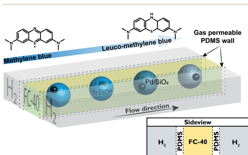
Fig. 1 Schematic representation of a polydimethylsiloxane (PDMS) microreactor with three parallel channels separated by 50 μm thick walls. H<sub>2</sub> can diffuse through the walls and hydrogenate methylene blue (MB) to leuco-MB in the presence of Pd/SiO<sub>2</sub> particles in ethanol droplets.
