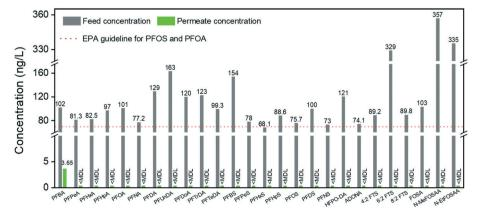
Fig. 6 PFAS treatment by the amyloid-carbon hybrid membrane
