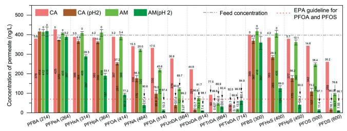
Fig. 1 Concentrations of PFCAs and PFSAs in the permeate. The pH of the feed is around 7 unless otherwise stated. The number in the brackets is the MW of each compound. The red dashed line stands for EPA guideline for PFOA and PFOS regulation, which is 70 ng  $L^{-1}$ . The grey dashed line stands for the spike concentration of each PFAS, which is around 400 ng  $L^{-1}$ . The removal efficiencies (%) are shown above the permeate bars.
