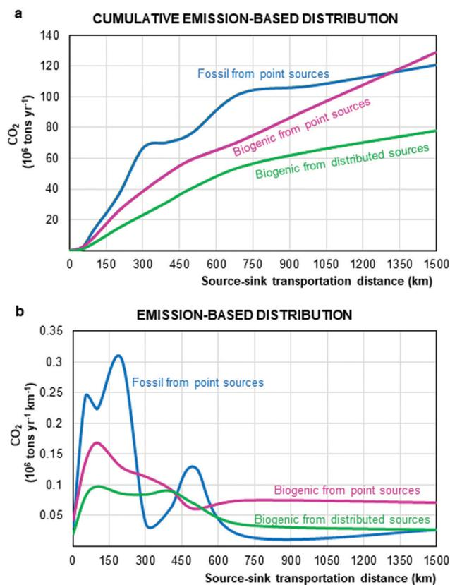
Fig. 6 Emission-based distribution of source–sink transport amount and distance of European CO<sub>2</sub>. (a) Cumulative emission-based distribution of source–sink CO<sub>2</sub> transportation distances from the 10 prospective CO<sub>2</sub> storage sites reported in Fig. 3. (b) Emission-based distribution of source–sink CO<sub>2</sub> transportation distances.
