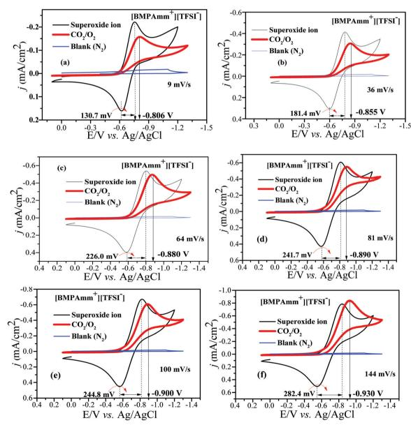
Fig. 5 (a-f) CVs of CO<sub>2</sub> conversion by O<sub>2</sub>• in [BMAmm<sup>+</sup>][TFSI<sup>-</sup>] after sparging with N<sub>2</sub> (background), CO<sub>2</sub>, O<sub>2</sub>, and CO<sub>2</sub>/O<sub>2</sub> simultaneously at 27 °C, GC vs. Ag/AgCl at various sweep rates.
