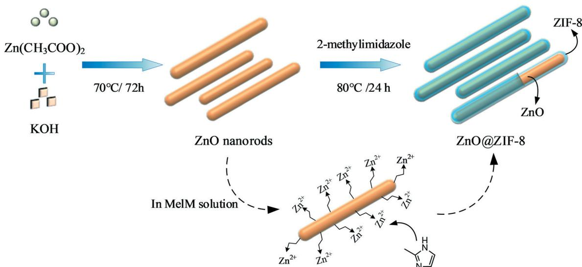
Fig. 1 Growth process of ZnO@ZIF-8 core-shell nanorods.
