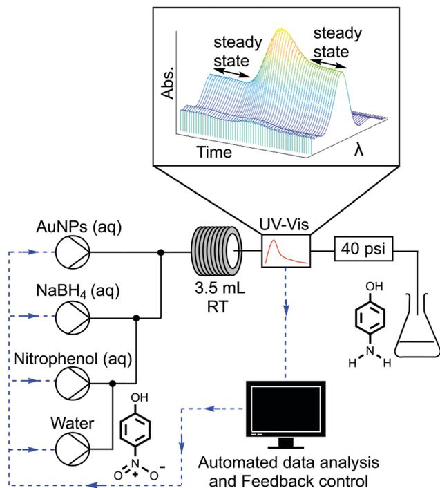
**Fig. 1** A schematic describing the self-optimising system. The experimental conditions are changed by altering the flow rates of the automated pumps, the reaction is monitored with an inline UV-vis spectrometer and optimised by closed-loop feedback control, based on the reaction conversion.
