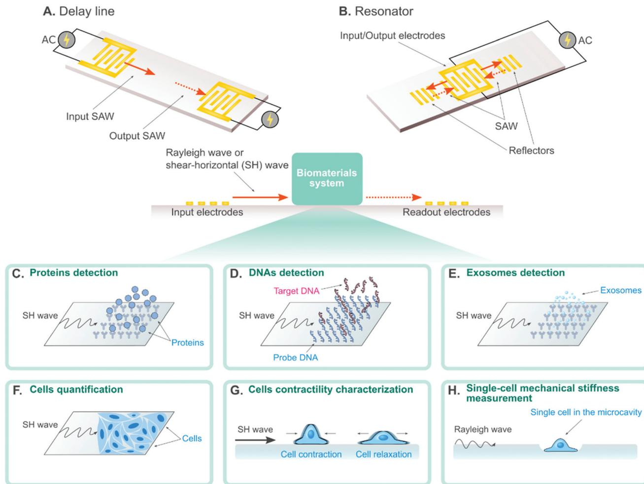
**Fig. 2** Schematic illustration of the working principles and representative applications of SAW sensors for biomaterials. Two different SAW sensors configuration include delay line (A) and one-port resonator (B) devices. Applications of SAW sensors for biomaterials include proteins detection (C), DNAs detection and analysis (D), exosomes detection (E), adherent cells quantification (F), cell contractility assessment (G), and single-cell stiffness analysis (H).
