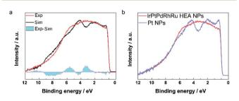
Fig. 3 (a) Comparison of the experimental VB spectrum of IrPdPtRhRu HEA NPs and the linear combination of VB spectra of the monometal NPs. The difference of the spectra is shown as cyan regions. (b) Comparison of the VB spectra of IrPdPtRhRu HEA NPs and Pt NPs.
