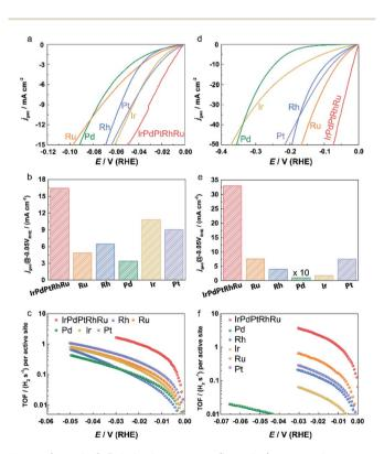
Fig. 4 (a and d) Polarization curves, (b and e) geometric current densities at an overpotential of 50 mV, and (c and f) TOF of IrPdPtRhRu HEA NPs and other monometallic catalysts in (a–c) 0.05 M  $\rm H_2SO_4$  solution and (d–f) 1.0 M KOH solution.
