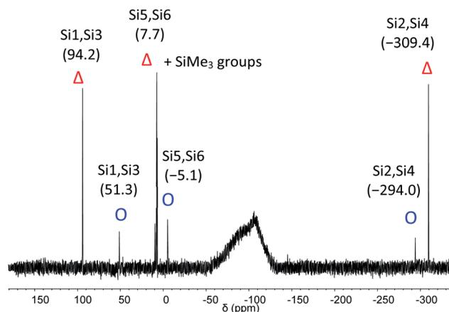
Fig. 3 <sup>29</sup>Si NMR spectrum of **2** in THF-*d*<sub>8</sub> at 210 K.  $\Delta$  represents the major component and O the minor component.
