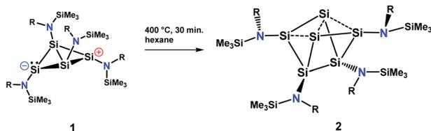
Scheme 4 Synthesis of the amido-substituted silicon cluster **2**.
