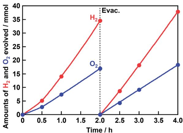
Fig. 4 Photocatalytic water splitting over  $\text{Rh}_{0.5}\text{Cr}_{1.5}\text{O}_3(0.2\text{ wt}\%)/\text{AgTaO}_3$  under UV irradiation. Photocatalyst: 1 g, reactant solution: distilled water (340 mL), cell: inner-irradiation cell made of quartz, light source: 400 W high pressure Hg-lamp.  $\text{AgTaO}_3$  was synthesized by a solid state reaction at 1273 K for 15 h without excess Ag.  $\text{Rh}_{0.5}\text{Cr}_{1.5}\text{O}_3$  was loaded by an impregnation method at 623 K for 1 h.
