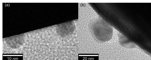
Fig. 2 TEM images of Rh<sub>0.5</sub>Cr<sub>1.5</sub>O<sub>3</sub>(0.2 wt%)/AgTaO<sub>3</sub> (a) before and (b) after photocatalytic water splitting under UV irradiation using a 300 W Xe-arc lamp. AgTaO<sub>3</sub> was synthesized by a solid state reaction at 1273 K for 15 h without excess Ag. Rh<sub>0.5</sub>Cr<sub>1.5</sub>O<sub>3</sub> was loaded by an impregnation method at 623 K for 1 h.
