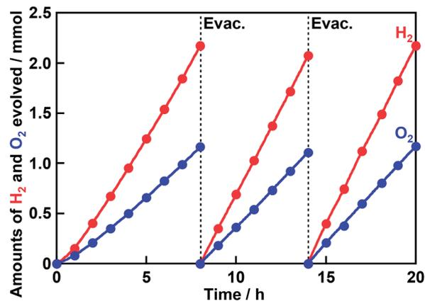
Fig. 1 Photocatalytic water splitting over Rh<sub>0.5</sub>Cr<sub>1.5</sub>O<sub>3</sub>(0.2 wt%)/AgTaO<sub>3</sub>. AgTaO<sub>3</sub> was synthesized by a solid state reaction at 1273 K for 15 h without excess Ag. Rh<sub>0.5</sub>Cr<sub>1.5</sub>O<sub>3</sub> was loaded by an impregnation method at 623 K for 1 h. Photocatalyst: 0.3 g, reactant solution: distilled water (120 mL), cell: top-irradiation cell with a Pyrex window, light source: 300 W Xe-arc lamp ( $\lambda > 300$  nm).
