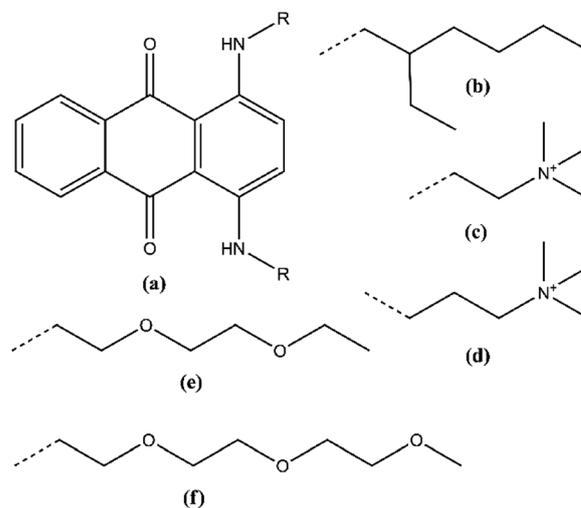
Fig. 1 Chemical structures of (a) 1,4-diaminoanthraquinone (DAAQ) and the side chains (R) on the amino positions: (b) 2-ethylhexyl (Et-He), (c) *N,N,N*-trimethylpropan-1-aminium (Me<sub>3</sub>N-Et), (d) *N,N,N*-trimethylpropan-1-aminium (Me<sub>3</sub>N-Pr), (e) 2-(2-(2-methoxyethoxy)ethyl) (Et-DEG), and (f) 2-(2-(2-methoxyethoxy)ethoxy)ethyl (Me-TEG). The dashed bonds represent the connection point of the side chains on the amino groups.
