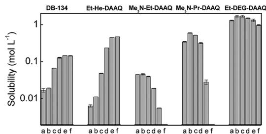
Fig. 3 Plot of the solubility (logarithmic scale) of the DAAQs in different solvent systems: (a) acetonitrile + 1 mol L<sup>-1</sup> TEATf<sub>2</sub>N, (b) acetonitrile/toluene 1/0, (c) acetonitrile/toluene 3/1, (d) acetonitrile/toluene 1/1, (e) acetonitrile/toluene 1/3, and (f) acetonitrile/toluene 0/1. Error bars are indicated at the top of the columns.
